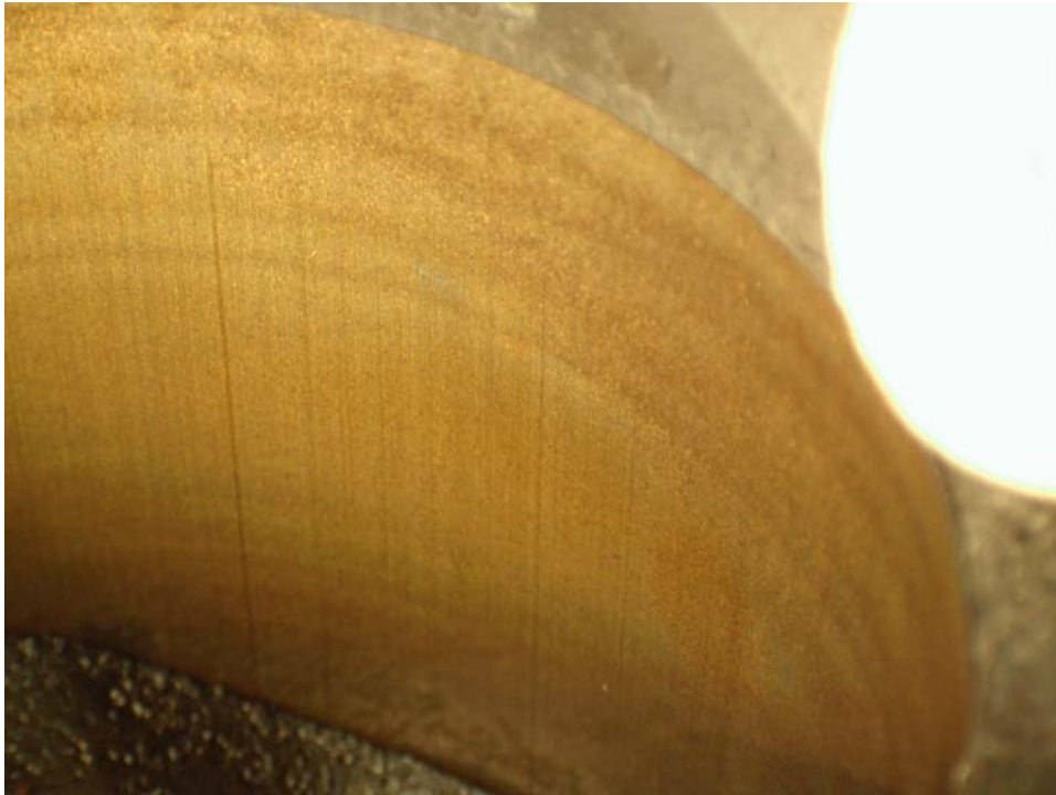
Figure 1 Corroded cylinder bore from an infrequently used Landrover in the NMA's collection. Note the horizontal banding, possibly due to contact with piston rings at rest. The vehicle was operated approximately three years prior to this image being taken.
